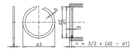
$\begin{array}{lll} b & = 4.00 \\ d1 & = 150 \\ d2 & = 152.6 \\ d3 & = 154.1 \\ Description = SB 150 \\ FN kN & = 102.00 \\ FR kN & = 36.20 \\ m min & = 2.7 \\ \end{array}$
